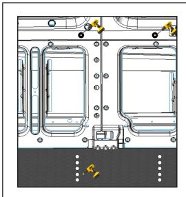
Drill all the marks using 3/8" drill bit.
