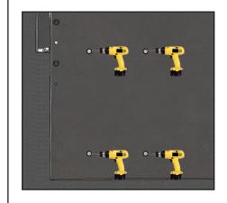
Drill all the marks using 3/8" drill bit.
