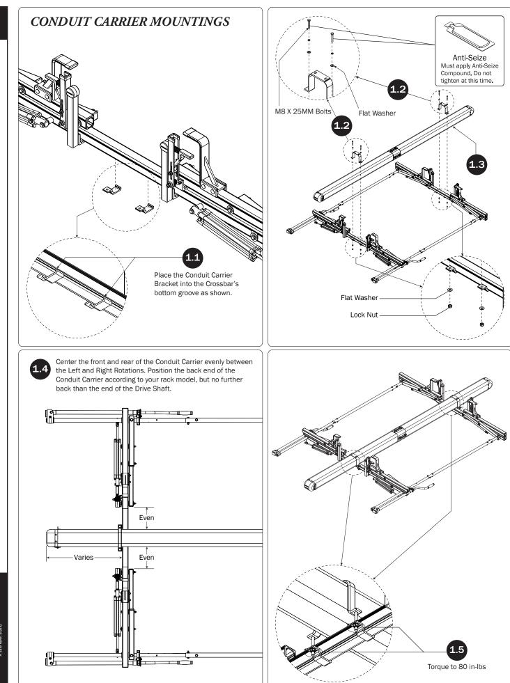
CON-8005 ASSEMBLY INSTRUCTIONS- GEN 4 CONDUIT CARRIER
