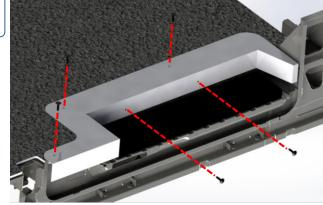
"Insert the five push-in rivets in the five holes drilled"
