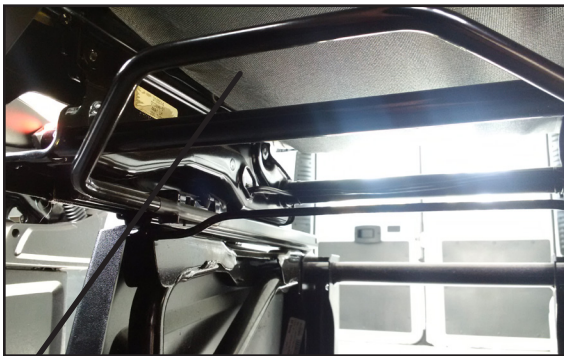
Seat cover bottom flap, running OVER all bars, wires, etc.
