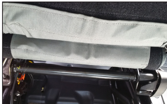
Seat cover bottom flap, running OVER all bars, wires, etc.
