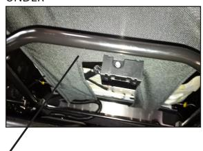
Seat cover bottom flap, running OVER all bars, wires, etc.
