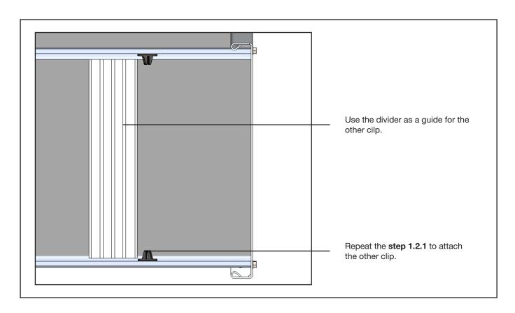
**1.2.3** After attaching the clips, slide the both ends of the divider to the clips.
