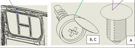
NOTE: DO NOT INSTALL HARDWARE IN THE HOLES AT THE TOP OF THE PANELS; THESE ARE USED FOR THE SILL INTALLATION. \*FOR ITEM 18, TOP SLIDING DOOR PANEL, ALIGN HOLES IN THE PANEL TO THE RIBS OF THE DOOR TO ENSURE PROPER SCREW INSTALLATION.
